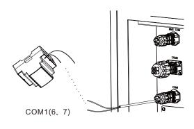
E. When connecting the smart meter to the inverter, connect one end of the cable to Terminal 13 (485B) and Terminal 14 (485A) of the smart meter and the other end to Pin 6 (485A) and Pin 7 (485B) of the COM1 port.
