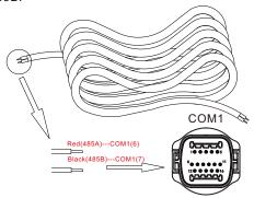
F. Dismantle the 16-pin connector delivered with the inverter and set aside the water-proof plug. Route the cables through each part sequentially, then connect them to Pin 6 and Pin 7. Finally, connect the connector to the COM1 port of the inverter.
