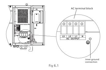
2>Firstly, unscrew the waterproof cover, then put the cable through the cover, pile the cable base on terminal size(17mm recommended), use a wire stripper to connect cable. and terminal, tighten all the terminal screws.
