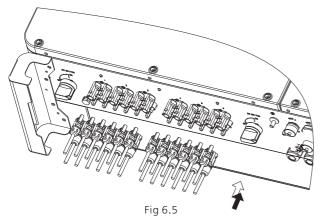
5>Decide the length of peeling base on cable terminal, use the wire stripper to connect cable and terminal, and separately connect to specific connector.
