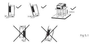
I. To ensure the inverter can work smoothly and easy for personnel to operate, please notice there is sufficient space for inverter, refer to following drawing.
