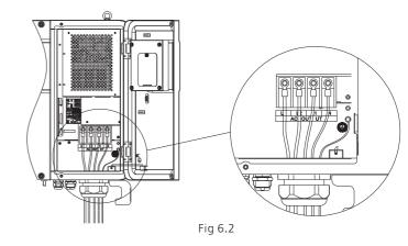
Diagram of how to install a terminal:
