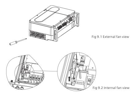
3>Disconnect the wire connector of the fans with a flat head screw driver and remove the fans from the fan guards, it is shown as below.
