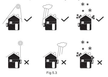
B. To reduce the de-rate performance of the inverter and extend inverter's life span, we strongly recommend you install an awning, for the distance between an awning and inverter, please refer to following drawing.
