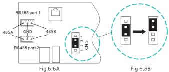
Notice: When multiple inverters are connected in parallel or the transmission distance is long, it is recommended to change the jumper cap of CN5 pin header on the Connector Board of the last inverter from the default 2/3 pin to 3/4 pin (As shown in Fig6.6B) . The reason for this is to increase the matching resistance.
