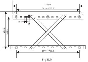
1>Use the wall mount plate as a template drill holes on the wall and put in expansion bolts.
