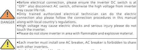
WARNING •It is forbidden to add load between inverter and breaker.
